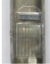
Figure 2: Wire type IQI
